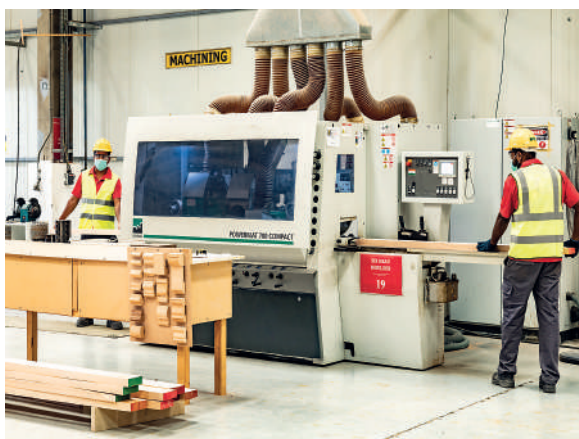
6 HEAD MOULDER WEINIG POWERMAT 700 MADE IN GERMANY
